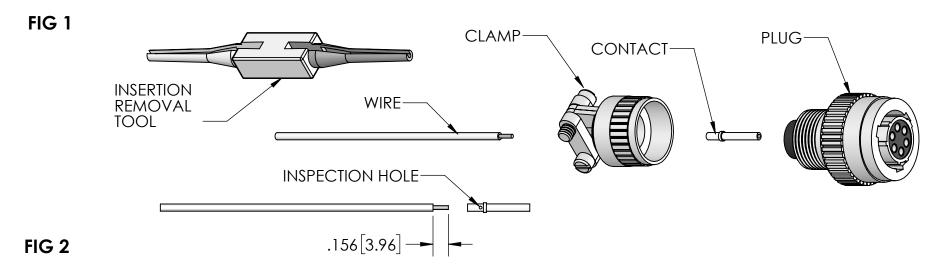
STRIP END OF WIRE TO DIMENSION SHOWN. INSERT WIRE FULLY INTO CONTACT, WIRE SHOULD BE VISIBLE IN INSPECTION HOLE. CRIMP WIRE TO CONTACT USING CRIMP TOOL SST P/N FP44440 AND LOCATOR SST P/N FP44441.
