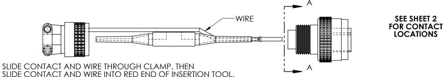
BEGINNING FROM THE CENTER CAVITY AND WORKING OUTWARDS IN A CIRCULAR PATTERN, INSERT WIRED CONTACTS INTO PLUG. (SEE FIG 4 (VIEW A-A) ON SHEET 2 FOR CONTACT LOCATIONS.) PUSH TOOL STRAIGHT INTO CAVITY UNTIL CONTACT SNAPS INTO POSITION. A LIGHT PULL ON THE WIRE WILL ASSURE THAT THE CONTACT IS SECURELY IN POSITION. REMOVE INSERTION TOOL AND REPEAT.
