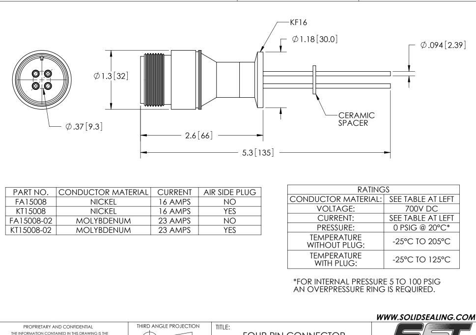
FOUR PIN CONNECTOR SOLE PROPERTY OF SOLID SEALING TECHNOLOGY, ANY REPRODUCTION IN PART OR AS A WHOLE WITHOUT THE WRITTEN PERMISSION OF SOLID SEALING TECHNOLOGY IS PROHIBITED. SOLID SEALING TECHNOLOGY, INC. REV. APP'D DATE SCALE 1:1 DRAWN MH 12/12/2006 DIMENSIONS IN PART NO. (SEE TABLE) REV. A INCHES [mm] MPDP0026-3ST ENG APPR. SALES DWG NO. FA15008SL REV. A3 A3 JS 11/26/2012 MH 12/12/2006
